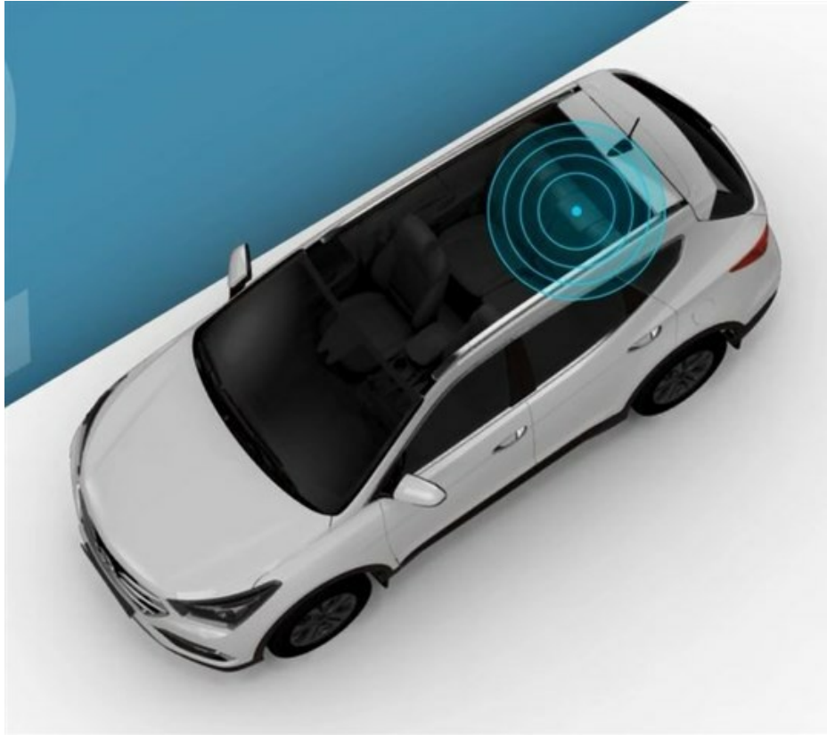
Ultrasonic sensors in the headliner of the vehicle detect movement in the rear seats
