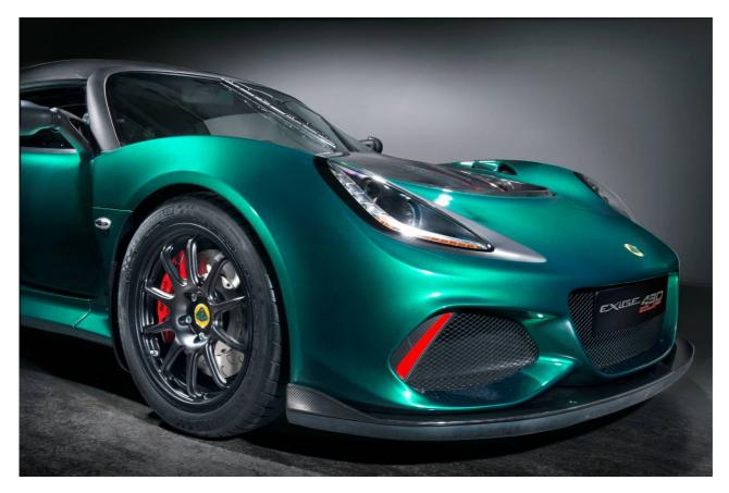
As you would expect, the intense use of ultra-lightweight carbon fibre only adds to the overall performance, as well as reinforcing the Exige Cup 430's physical presence. The hand-made composite components include front splitter, front access panel, roof, diffuser surround, large aperture air-intake side pods, one-piece tailgate and the race derived rear wing.
